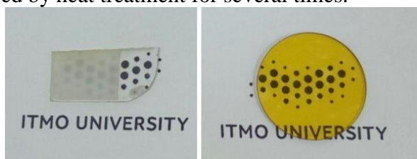
Figure 1. Daylight photo of the PTR matrix-based glass (left) and BK-7 Schott glass (right) after \text{Na}^+ - \text{Ag}^+ IE and heat treatment. Silver nanoisland film on the PTR glass surface is partially removed.
